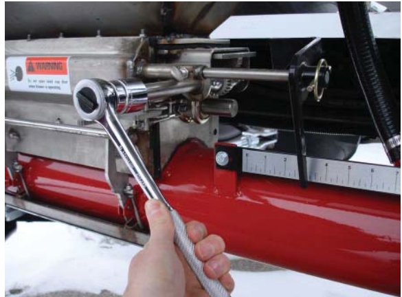
Adjusting the Meter Gate
