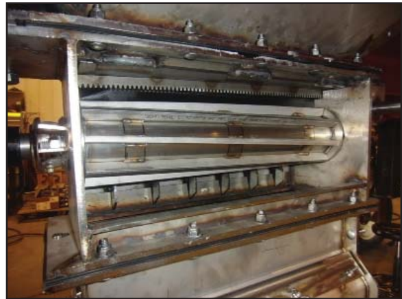
The meter with door removed
