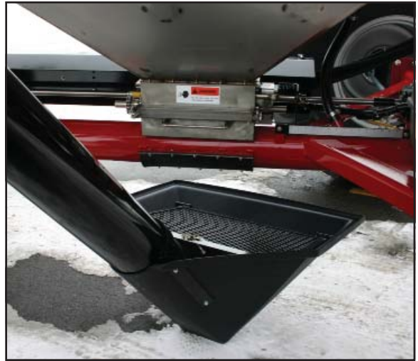
Placing the hopper under the meter
