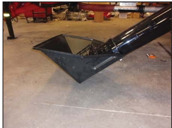
Hopper in the upright position
