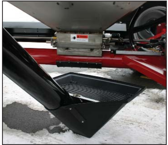
Placing the hopper under the meter
