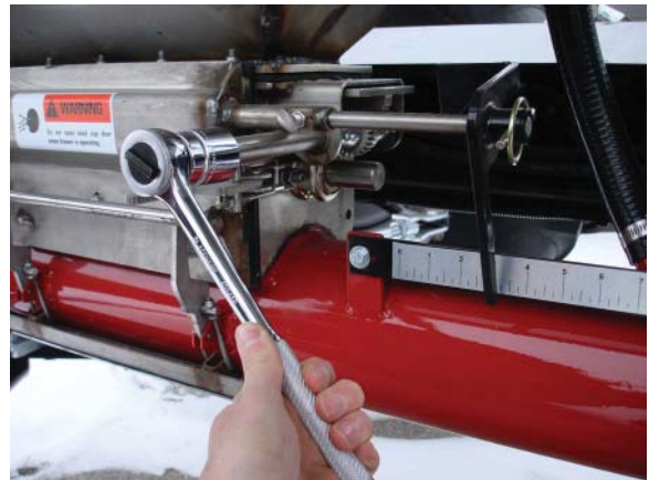
Adjusting the Meter Gate
