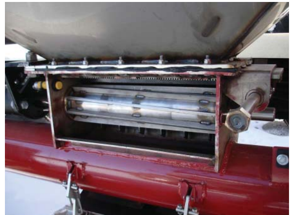
The meter with door removed
