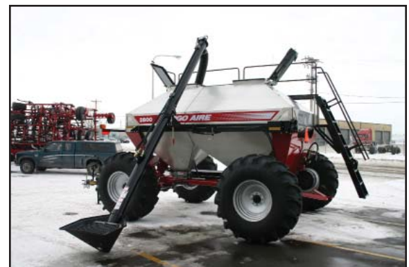
Air cart with auger in loading position
