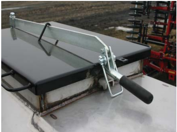
Lid and latch with toggle u-bolt adjustment
