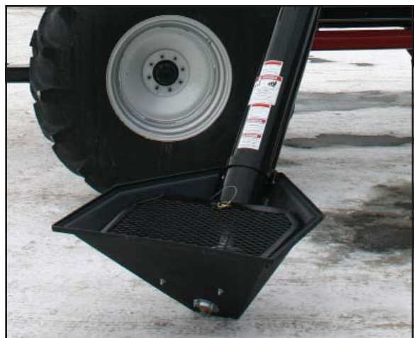
Hopper in the upright position
