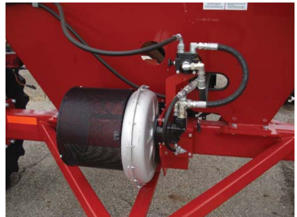
The blower and associated hydraulics
