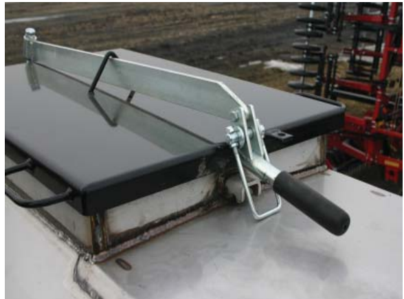
Lid and latch with toggle u-bolt adjustment
