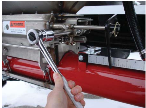
Adjusting the Meter Gate
