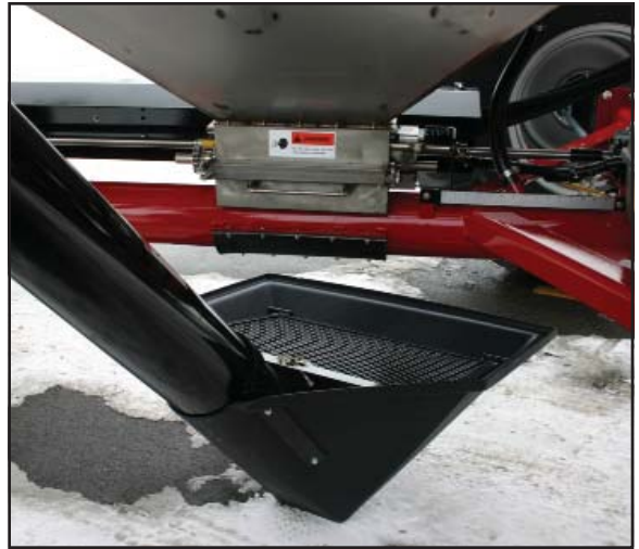
Placing the hopper under the meter
