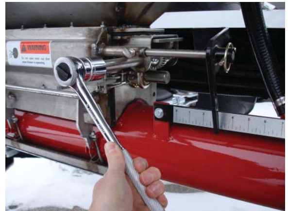
Adjusting the Meter Gate
