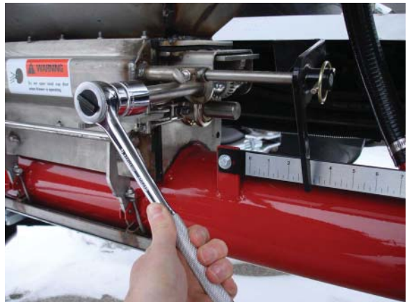
Adjusting the Meter Gate
