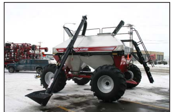
Air cart with auger in loading position
