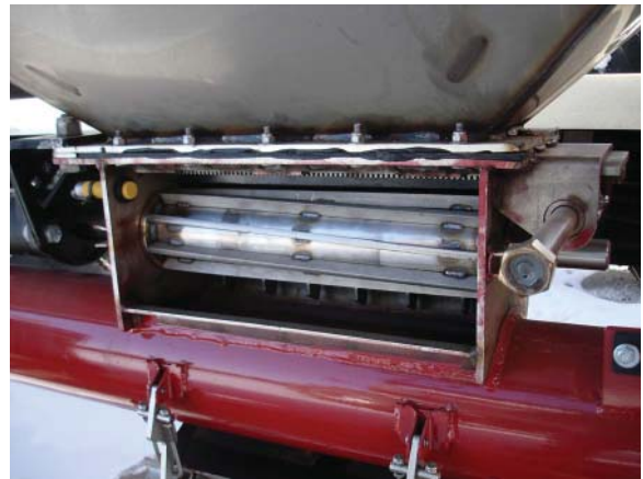
The meter with door removed
