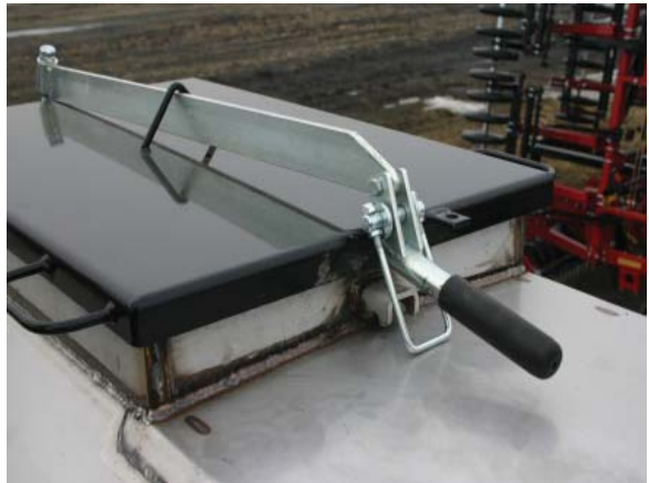
Lid and latch with toggle u-bolt adjustment
