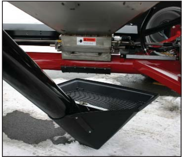
Placing the hopper under the meter
