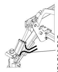
NOTE: CYLINDERS ON FRONT LIFT AXLES AND REAR PACKER LIFTS MUST BE MOUNTED WITH RODS UP AND PORTS TO THE SIDE. REMOVE AND ROTATE END GLANDS IF REQUIRED. FAILURE TO ORIENTATE AS INDICATED CAN CAUSE PORT INTERFERENCE, CHECK FOR INTERFERENCE BEFORE AND WHILE ACTIVATING ALL CYLINDERS.
