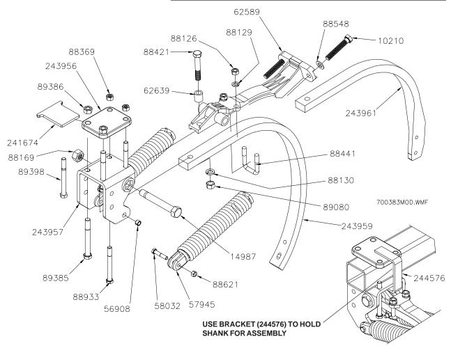
89398 BOLT USED WITH 241764 SHIM AND 241675 SHIM KIT
