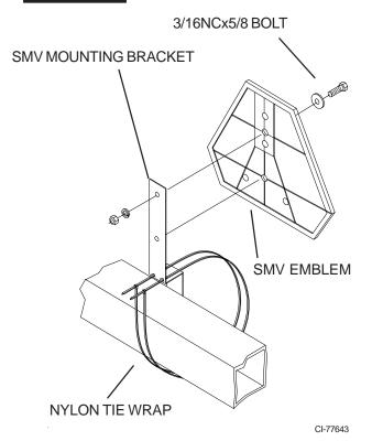
The bracket provided is designed to mount to numerous frame sizes and can be orientated in numerous positions to avoid interference with implement components.
