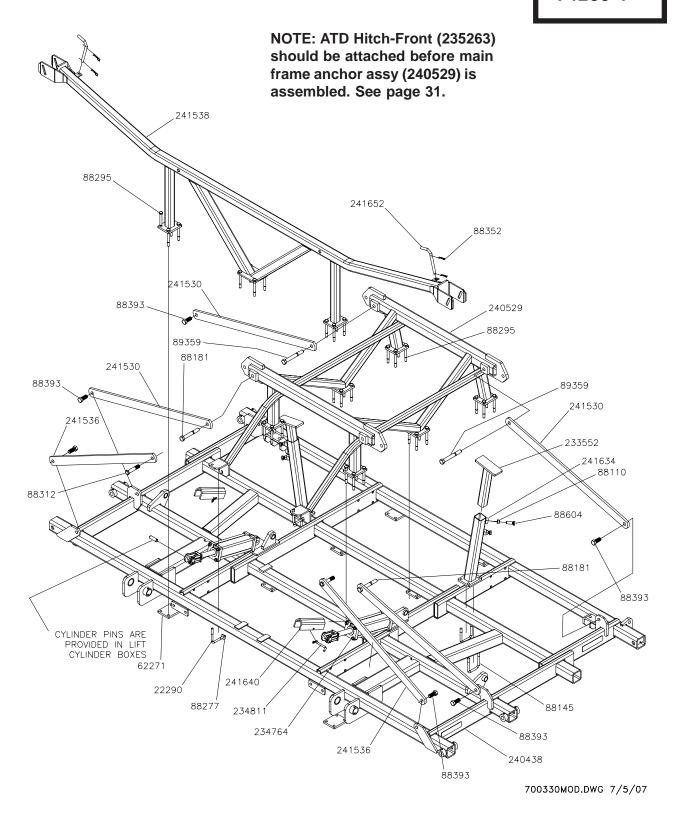
UNLESS SPECIFIED, ALL HARDWARE IS SECURED WITH MATCHING LOCK NUTS
