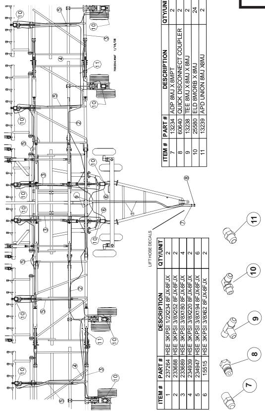
Hose are equipped with JIC fittings, tighten to seal, do not overtighten. Cylinder port require O-ring fittings, tighten to compress the O-ring to seal. Pipe thread fitting require some type of thread sealant to seal.
